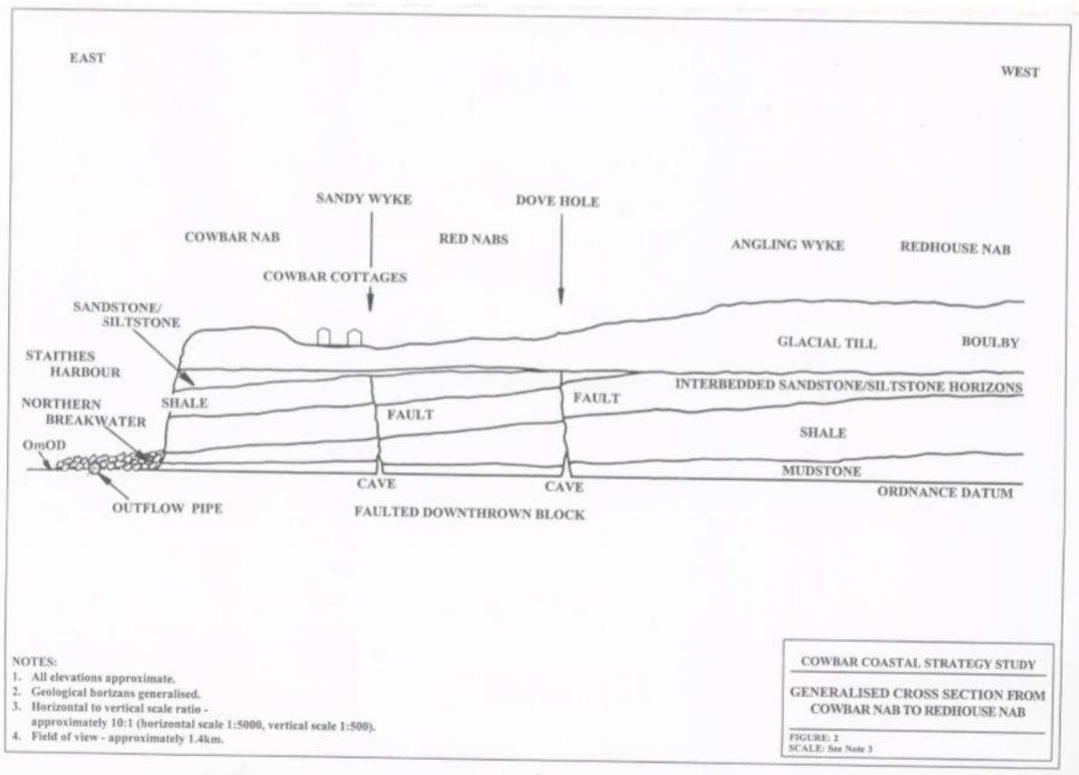
**Figure 1 – Generalised Cross Section from Cowbar Nab to Redhouse Nab**
